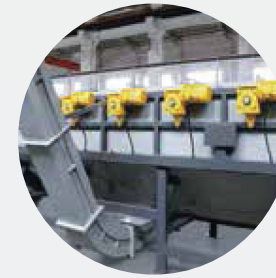
Float-sink Washing Tank
