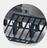
Automatic feeding flip - Hydraulic powered feeding flip for loading heavy and large diameter pipes
